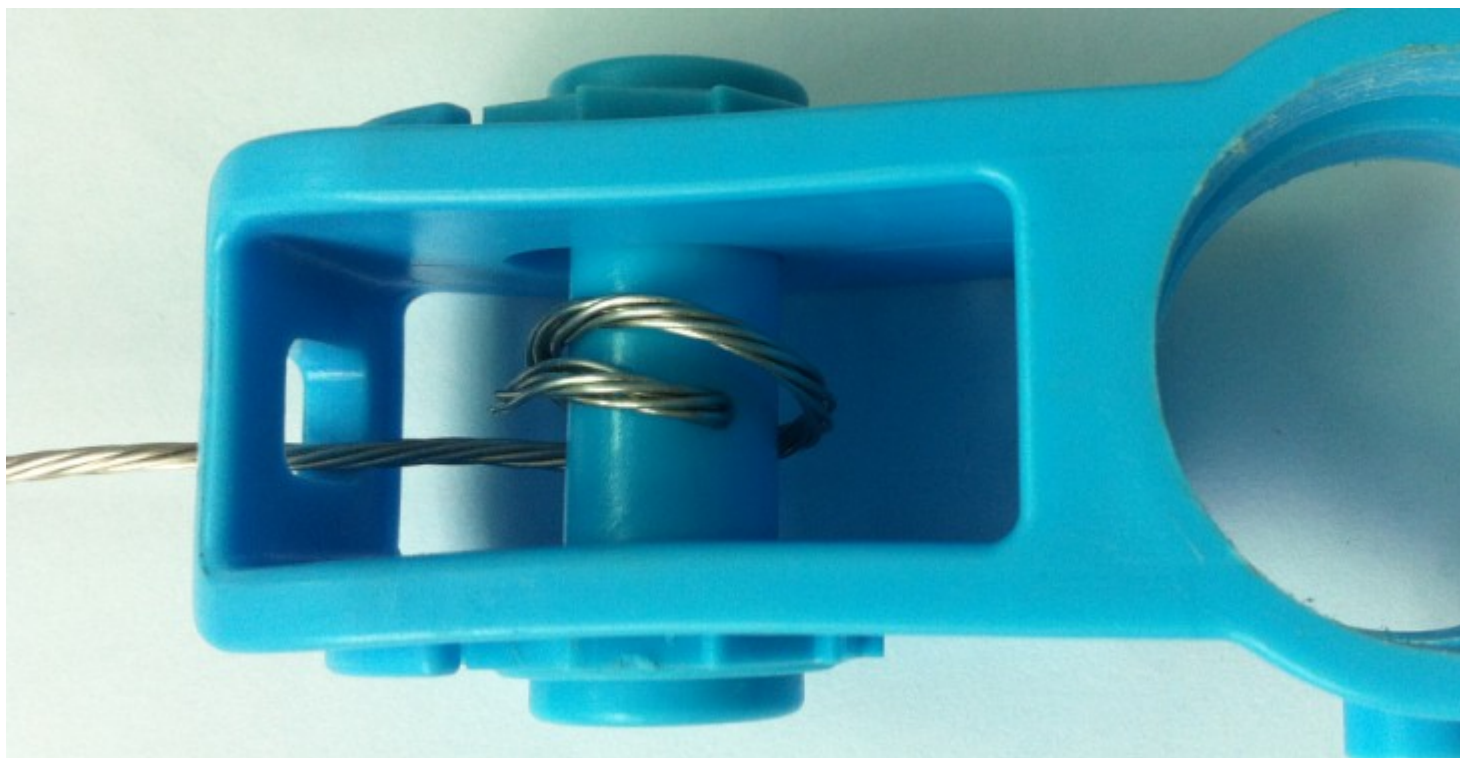
用内六角扳手拧终端杆绝缘子侧边的卡位，收紧合金线 Screw one side of the terminal rod insulator by inner hex key to tighten alloy wire
